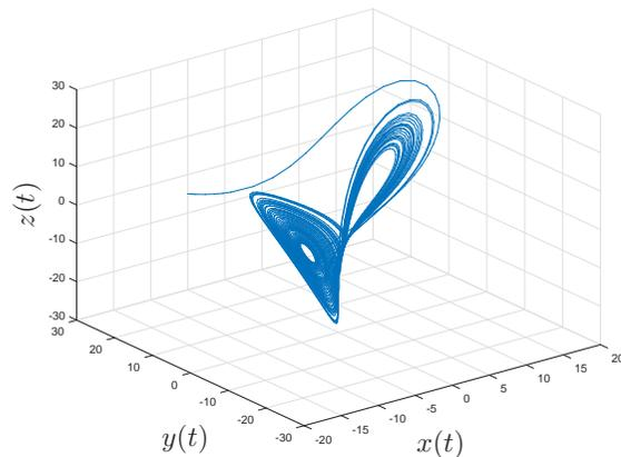
$$\begin{aligned} \dot{x}(t) &= \sigma(y(t) - x(t)) \\ \dot{y}(t) &= rx(t) - y(t) - x(t)z(t) \\ \dot{z}(t) &= x(t)y(t) - bz(t) \end{aligned}$$
