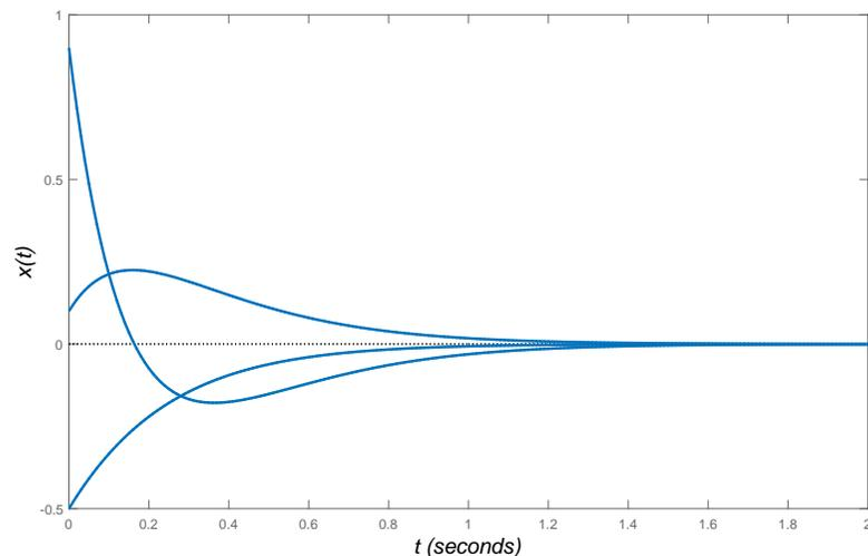
$$\xi = 1 : x_h(t) = (x_0 + (v_0 + \omega_n x_0)t)e^{-\omega_n t}$$
