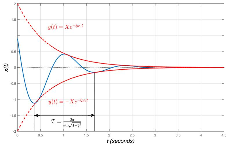
$$X = \sqrt{x_0^2 + \left( \frac{\xi\omega_n x_0 + v_0}{\omega_n \sqrt{1-\xi^2}} \right)^2}$$
