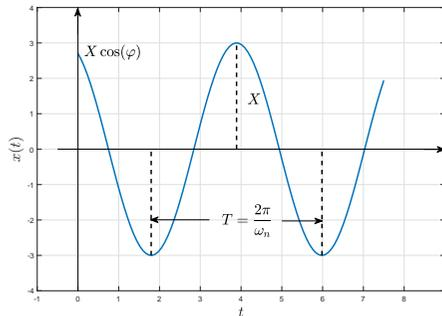
$$x_h(t) = \frac{v_0}{\omega_n} \sin(\omega_n t) + x_0 \cos(\omega_n t) = X \cos(\omega_n t + \varphi)$$
